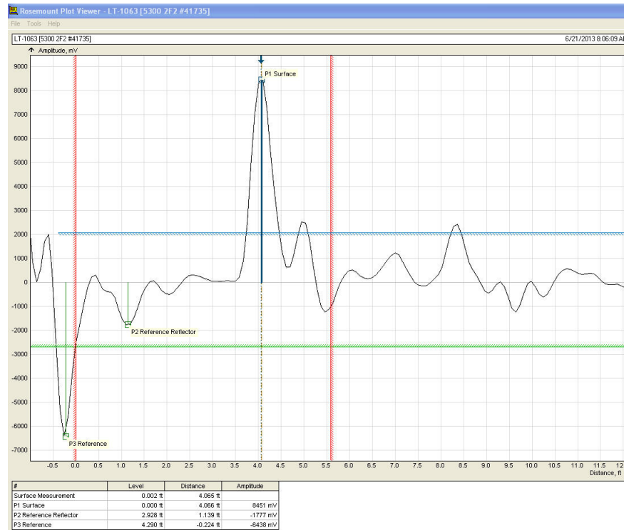
Figure 5-3. Rosemount 5300 Series with DVC - Echo curve presentation in RRM
